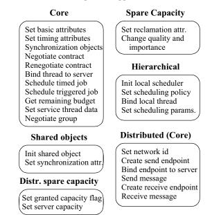
Figure 3. Main elements of the FSF API
