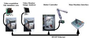
Figure 6. Industrial robot controller implemented with distributed FSF
